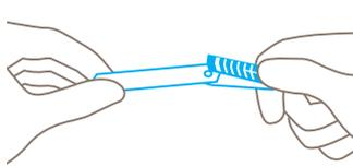
Lift the slider, take out and change the blade, then position the new blade **exactly on the cam**. For left hand use, turn blade over. The two magnets fix the blade additionally.
