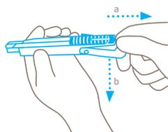
Pull the blade change button to the back as marked by the arrow (a), flip the end of the handle downwards (b) and **move the blade out of the handle** by using the slider.
