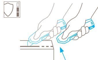
**Fully automatic blade retraction – a very high degree of safety**
