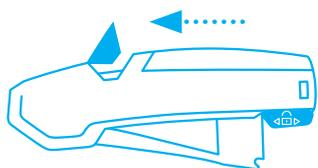
Pull the **blade change button** to the top and release the lever. Blade and blade holder will come out of the handle.
