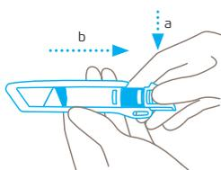
Press the blade change button and remove the plastic insert from the rear of the handle.
