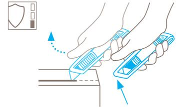
**Automatic blade retraction – a high degree of safety**
