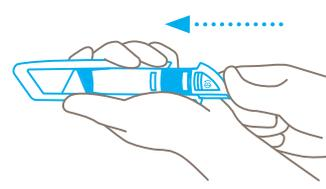
Close the blade cover and push the plastic insert back into the handle until the blade change button **audibly** clicks.
