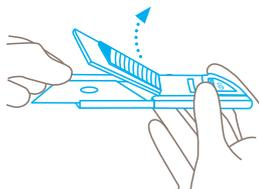
Hold the **blunt** side of the blade and use it to lift the blade cover upwards. The cover remains in the open position.
