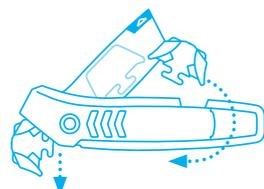
Remove the fitted blade from the head of the cutter. Now you can either **rotate or replace** the blade.
