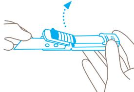
Hold the **blunt** side of the blade and use it to lift the blade cover upwards. The cover remains in the open position.
