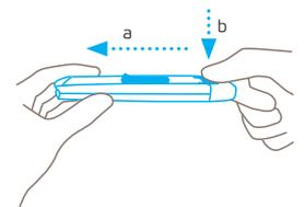
Close the blade cover and push the plastic insert back into the handle and then **press down** on the blade change button.
