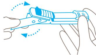
Replace the blade. Make sure you place the blade **exactly on the locating lobes**. Left-handers turn the blade 180°.
