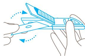
Reverse or replace the blade. Make sure you place the blade **exactly** on the locating lobe.
