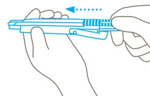
At last, slide the inner part with the blade **back into the handle** and flip the end of the handle upwards. Release and snap back the blade to ensure flawless functionality.
