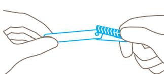
Lift the slider, take out and change the blade, then position the new blade **exactly on the cam**. For left hand use, turn blade over. The two magnets fix the blade additionally.
